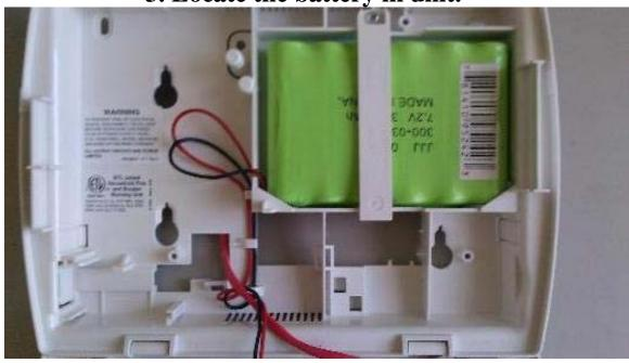
4. Locate and disconnect the battery lead from the mother board by gently unplugging the wire from the terminal on the board
